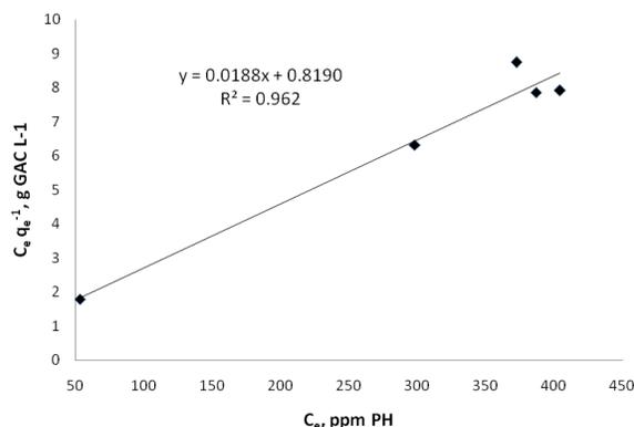
Fig. 4. Linear transformation of the adsorption isotherm for PH on GAC prepared with R= 2 from CNs using the Langmuir model.
