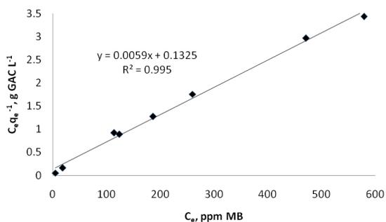
Fig. 3. Linear transformation of the adsorption isotherm for MB on GAC prepared with R= 2 from CNs using the Langmuir model.
