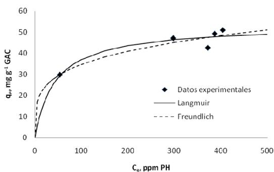
Fig. 2 Adsorption isotherm for PH on GAC prepared with R= 2 from CNs
