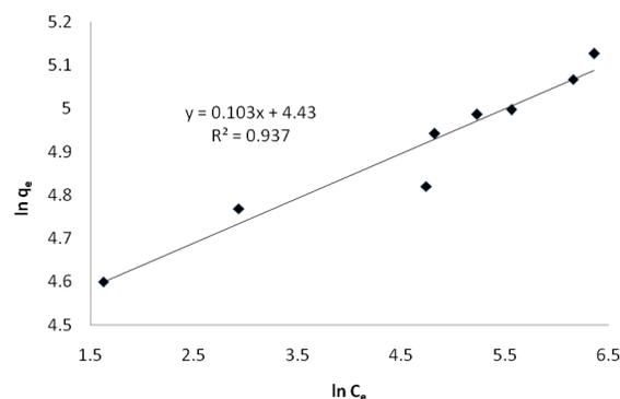
Fig. 5. Linear transformation of the adsorption isotherm for MB on GAC prepared with R= 2 from CNs using Freundlich's model.
