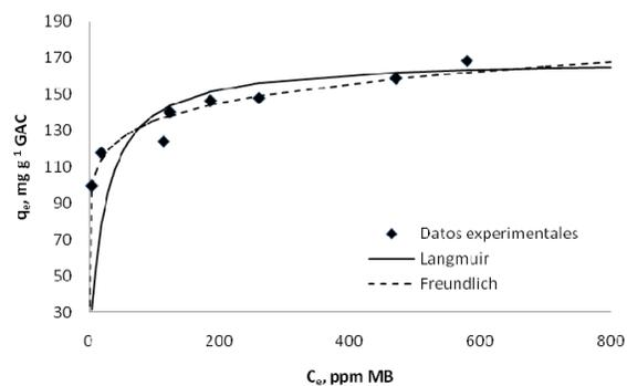
Fig. 1 Adsorption isotherms for MB on GAC prepared with R= 2 from CNs
