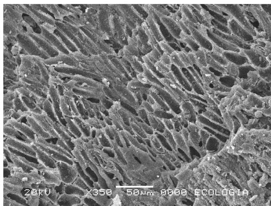
Image 2. GAC surface porosity. Scale line equals 50 μm.
