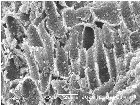
Image 3. Internal porosity of GAC produced from PN with R=2.
